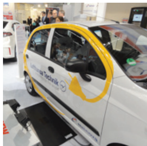
An example of inductive charging from Frankfurt. The vehicle positions itself above the pad on the ground to complete the connection (the above pad is offset for illustrative purposes)
