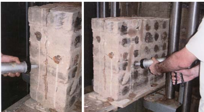
Fig. 19 Testing masonry models after grouting with soil grouts After testing the results were compared with sound masonry models.
