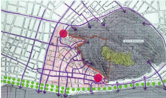
The image is to be considered a diagram of the problems which characterize the role of the city centre: few connections, scarce access to the port and to the hill, too big buildings which border the district and separate it from the other parts of the city
